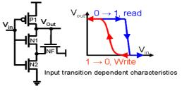
Figure 2: Schmitt Trigger Principle
