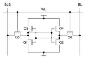
Figure 1: Conventional 6T SRAM Cell
